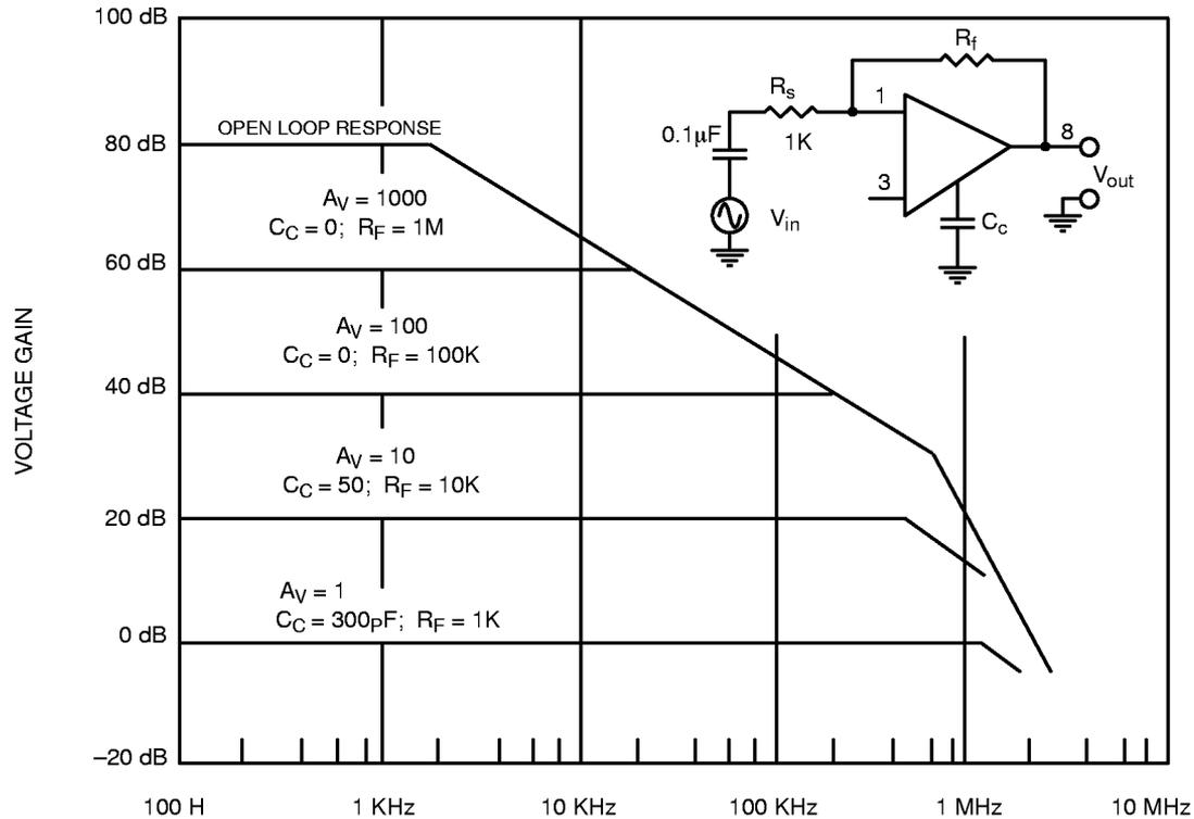
**Figure 11. XR-215 Op Amp Frequency Response**
