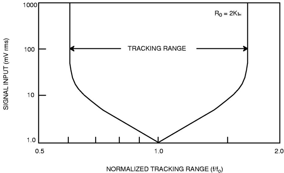
**Figure 26. Tracking Range vs Input Amplitude (Pin 10 Open Circuited)**
