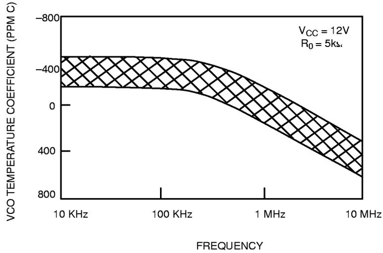
**Figure 7. Typical VCO Temperature Coefficient Range as a Function of Operating Frequency (Pin 10 open)**
