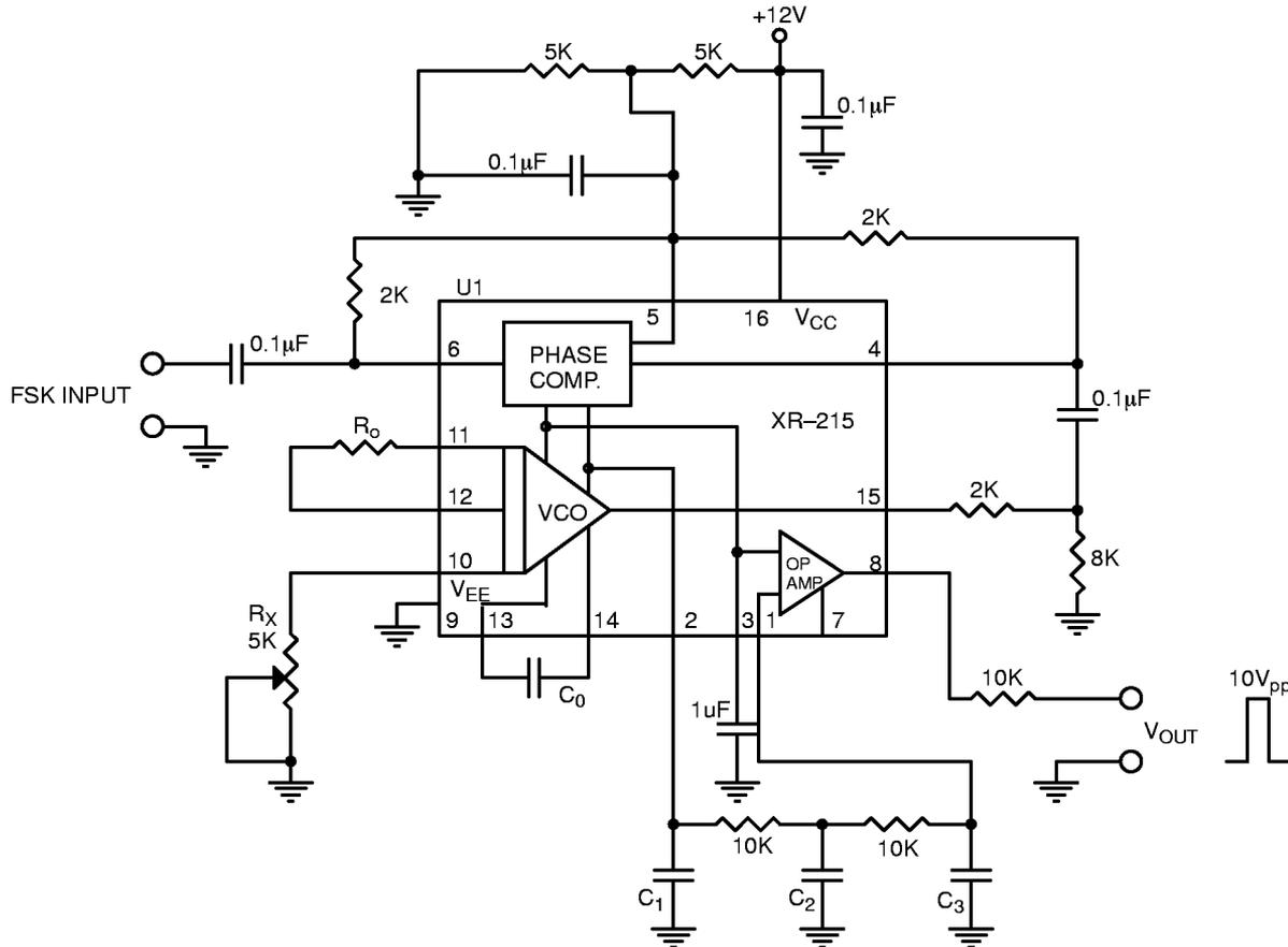
**Figure 21. Circuit Connection for FSK Demodulation**
