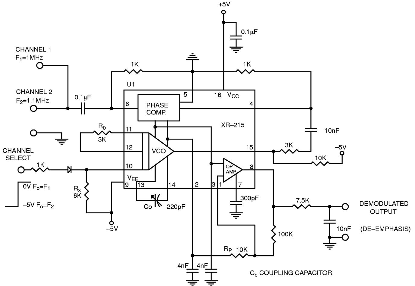
Figure 19. Time-Multiplexing XR-215 Between Two Simultaneous FM Channels
