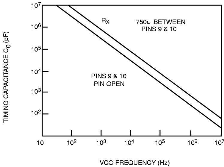
**Figure 8. VCO Free Running Frequency vs. Timing Capacitor**
