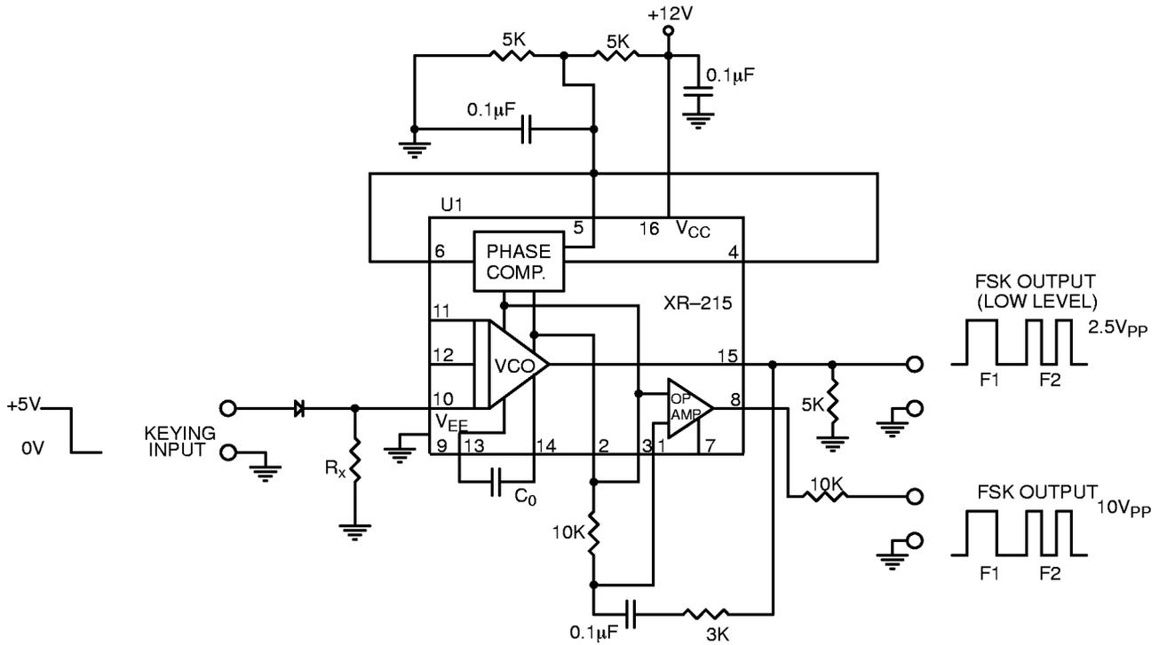
Figure 22. Circuit Connection For FSK Generation
