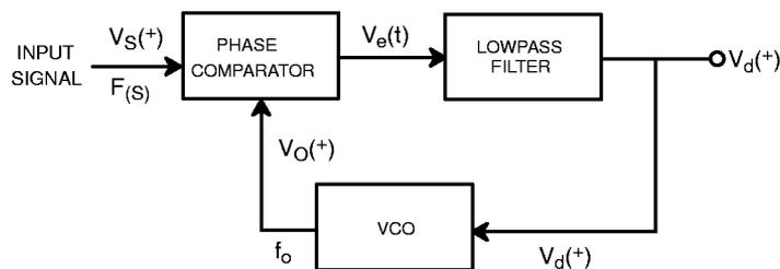
Figure 13. Block Diagram of a Phase-Locked Loop
