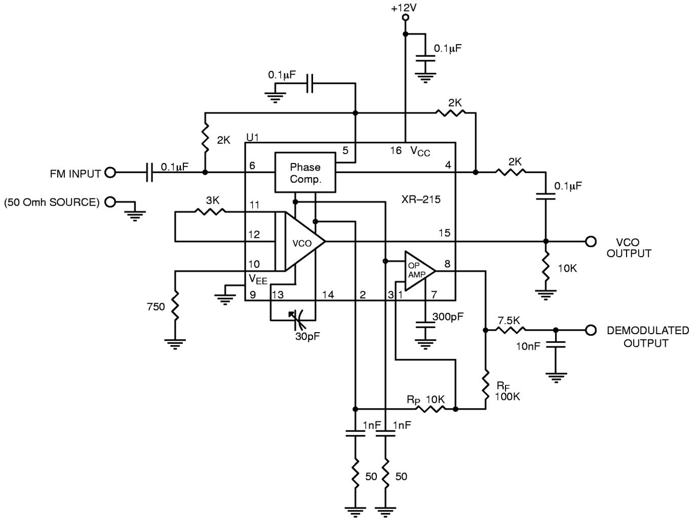
**Figure 5. Test Circuit for FM Demodulation**
