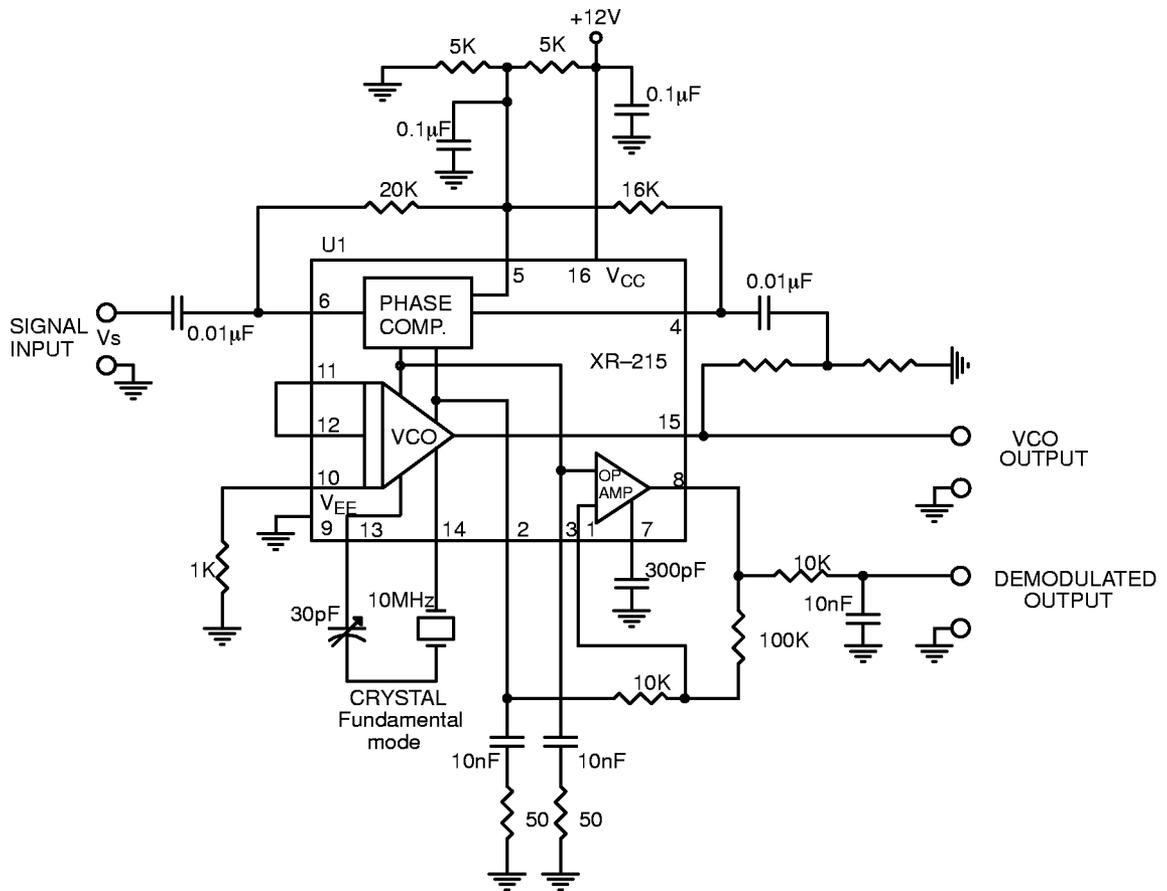
Figure 28. Typical Circuit Connection for Crystal-Controlled Clock Recovery.
