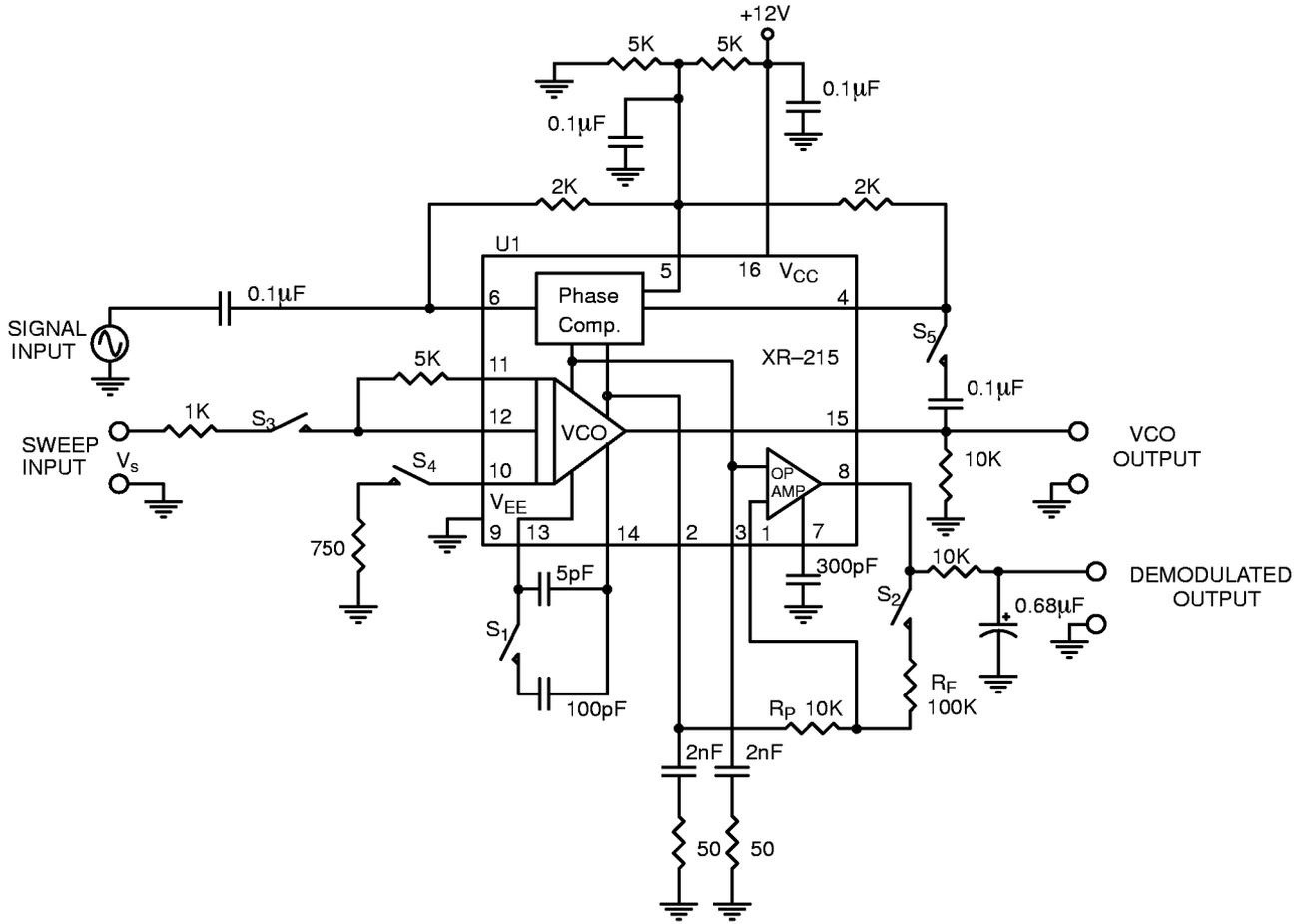
**Figure 3. Test Circuit for Single Supply Operation**
