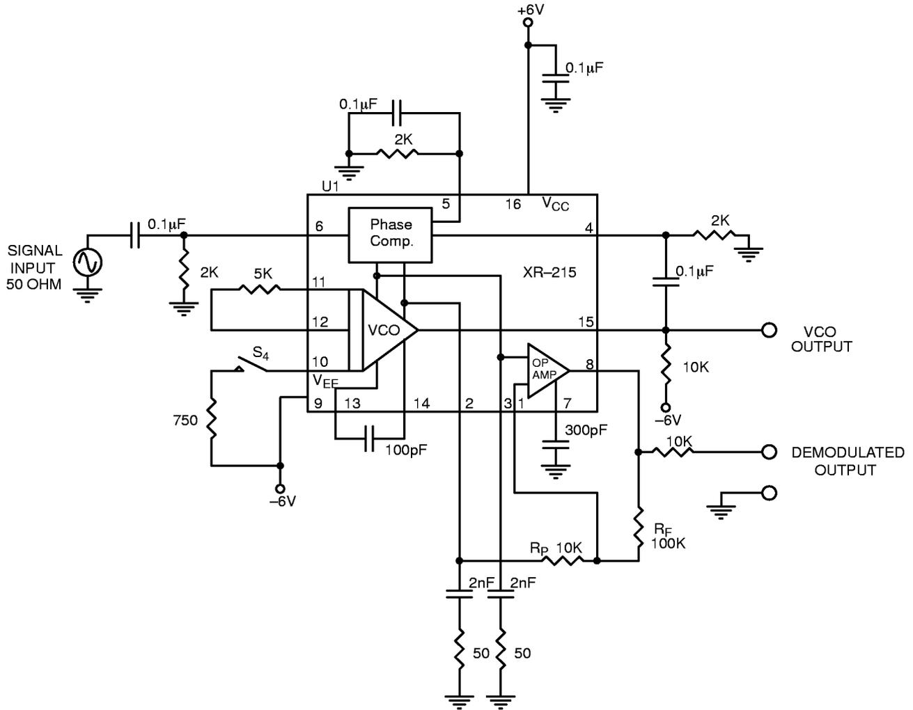
Figure 4. Test Circuit for Split-Supply Operation
