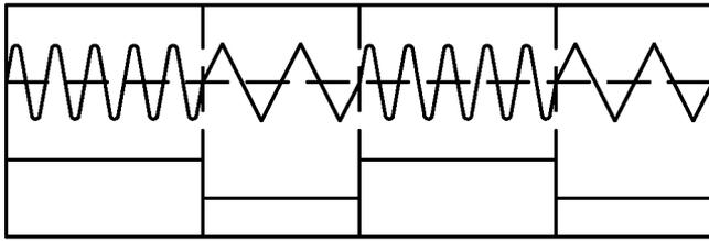
**Figure 20. Demodulated Output Waveforms for Time-Multiplexed Operation**
