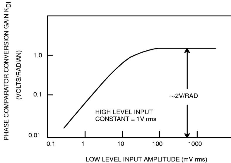
Figure 9. Phase Comparator Conversion Gain,  $K_d$ , versus Input Amplitude
