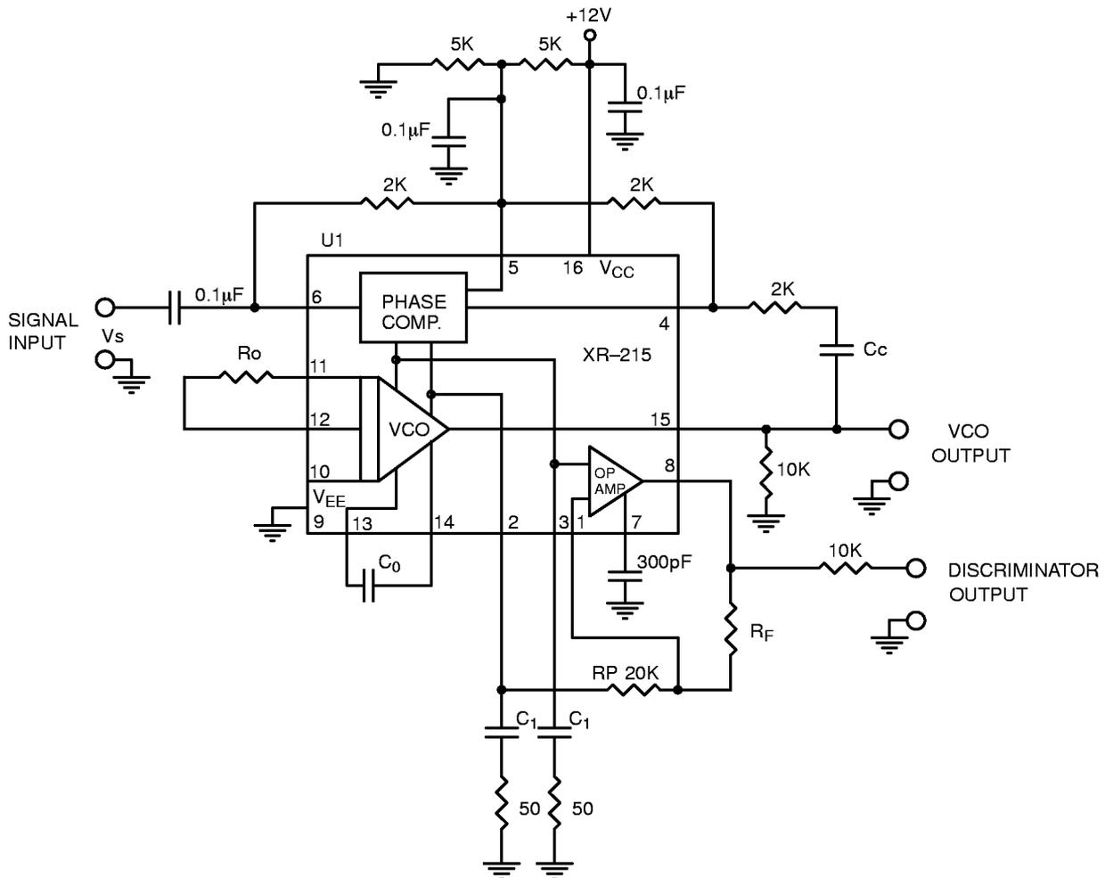
Figure 25. Circuit Connection For Tracking Filter Applications
