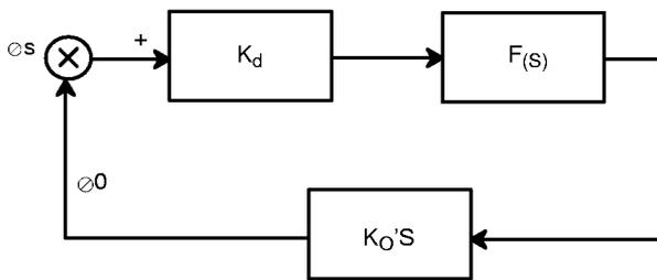
**Figure 14. Linearized Model of a PLL as a Negative Feedback System**
